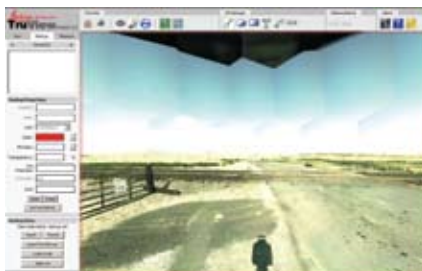
Above: A laser scan point cloud of the railroad crossing. Below: A screen shot of a 180-degree laser scan overlaid on a digital photo.
