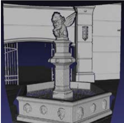
Top Left: A colored point cloud with a digital photo overlay. Above: A point cloud of a statue based on scan density and reflectivity of the material surface.
