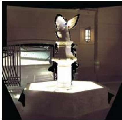
Top Left: A colored point cloud with a digital photo overlay. Above: A point cloud of a statue based on scan density and reflectivity of the material surface.
